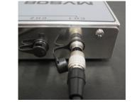
4-3 Connecting the preamplifier UPT01 and Mold Surface-Temperature Sensor Connect the mold surface temperature sensor to the preamplifier UPT01. (The thicker side metallic terminal width of sensor is the center side of UPT01.) Insert the sensor connector into UPT01 connector as far as it will go. Hold UPT01 firmly when removing the sensor,
