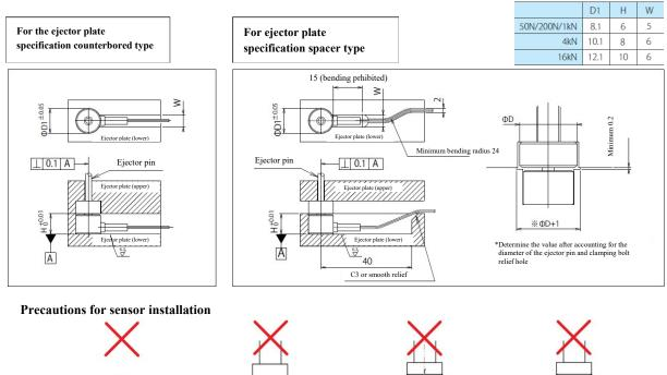
R Do not machine the bottom with round edges
