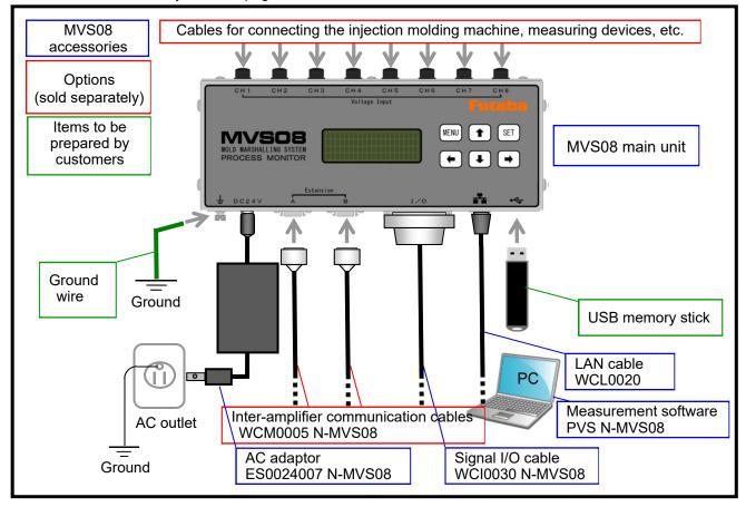
As shown in the above figure, "MVS08" is structured to connect measuring devices with dedicated cables.
