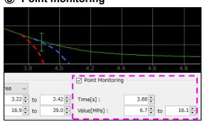
Blue dotted waveform: OK Red dotted waveform: Alarm
