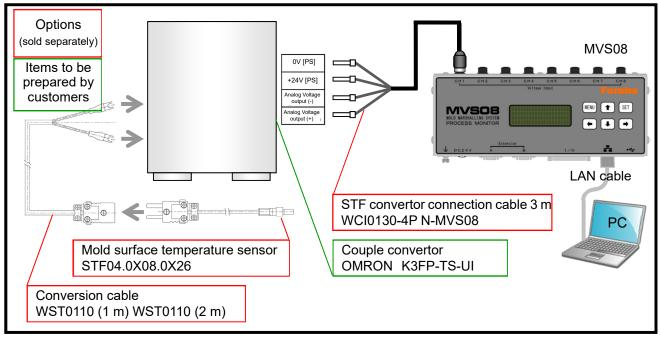
(7) When connecting other manufacturers' measuring devices and an injection molding machine, etc. ....For the connection of the MVS08 side, see paragraph (1) on Page 13.
