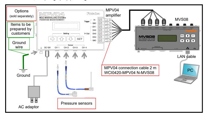
(4)When connecting a inline injection resin pressure measuring unit "MPS01A" ···· For the connection of the MVS08 side, see paragraph (1) on Page 13.
