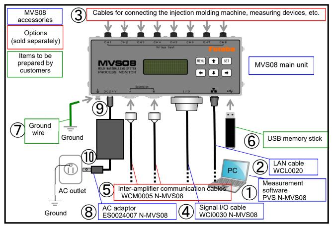
① Install the measurement software. ②Connect the LAN cable.
