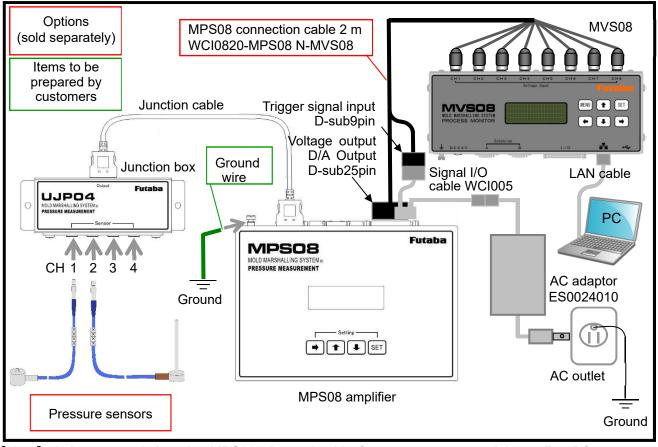
[Note] It is assumed that the MPS08 shown in this figure operates standalone. For PC-connected operation, a PC is required separately. The MPS08 can store measurement condition setting files. To change the measurement conditions, however, it needs to be connected to a PC.
