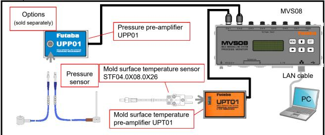
(9) When connecting additional injection molding monitoring system "MVS08" units to a "MVS08 set"
