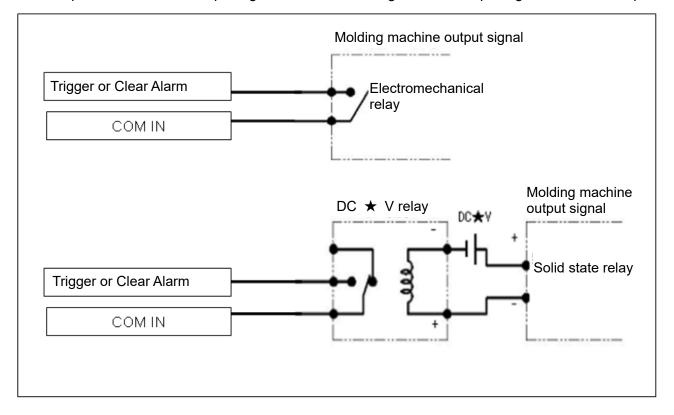
Example 2: When the output of the molding machine connected to the main unit is "voltage output" Connect the signal by using a relay adaptable to the output voltage of the output signal from the molding machine.
