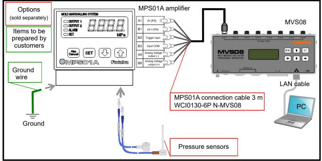
[Note] No power cable nor AC adaptor is required as power is supplied from MVS08 via MPS01A connection cable.
