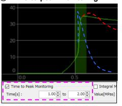
Blue dotted waveform: OK Red dotted waveform: Alarm
