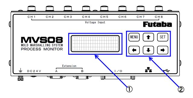
Display panel ..... Displays the status of measurement, setting file name, shot counter, and set conditions, file name and setting status in the main unit, etc.
