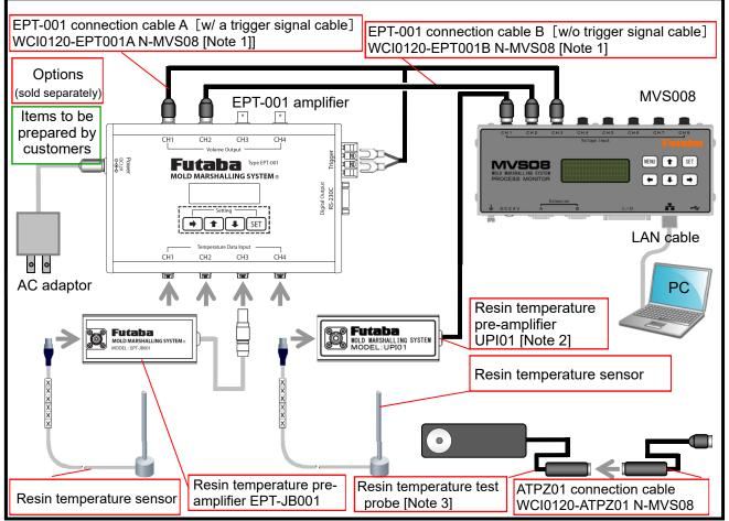
[Note 1] EPT-001 connection cable A is used for the connection of EPT-001 CH1. Trigger signals can be captured. EPT-001 cable B is used for the connection of EPT-01 CH2 to CH4. Only voltage signal can be captured.
