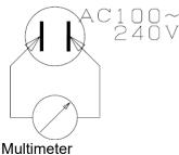
(2) Using a multimeter, measure the voltage between each terminal of the AC power outlet and the ground to make sure that one is 0 V and the other is AC100 to 240V.
